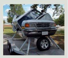
The rollover crash simulator demonstrates what can happen to passengers if they are not buckled up. Dummies are placed into a rotating truck cab. At first, seatbelts are used and the dummies remain in the truck. When the seatbelts are removed, the dummies are thrown from the truck.
