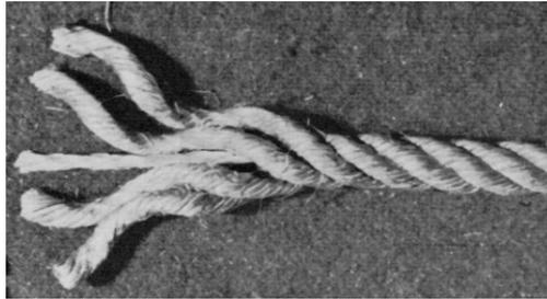
Shroud-laid rope has four strands laid up right-handed around a heart or core.
